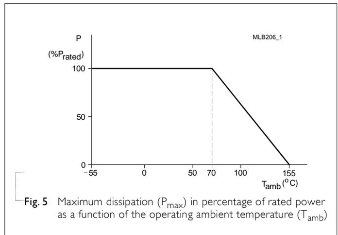
Fig. 5 Maximum dissipation (P<sub>max</sub>) in percentage of rated power as a function of the operating ambient temperature (T<sub>amb</sub>)
