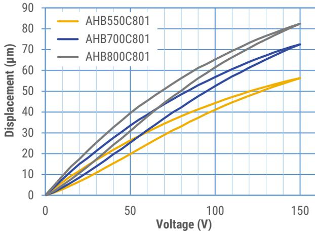
Figure 2 - Voltage vs. Displacement- 2
