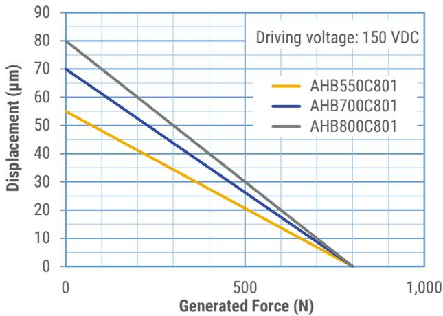
Figure 4 - Generated Force vs. Displacement- 2
