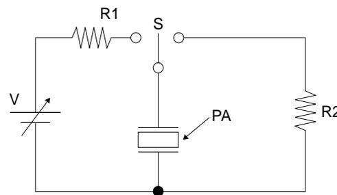
Protective resistor  $R1=1k\Omega$
