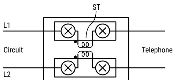
② Insertion in Driver/Receiver circuit in telephone
