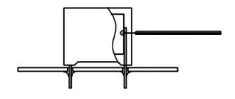
Temperature monitored inside the capacitor.
