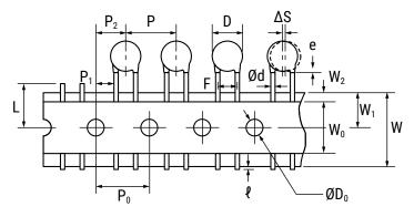
5 mm, 7.5 mm, 10 mm and 12.5 mm Lead Spacing:
