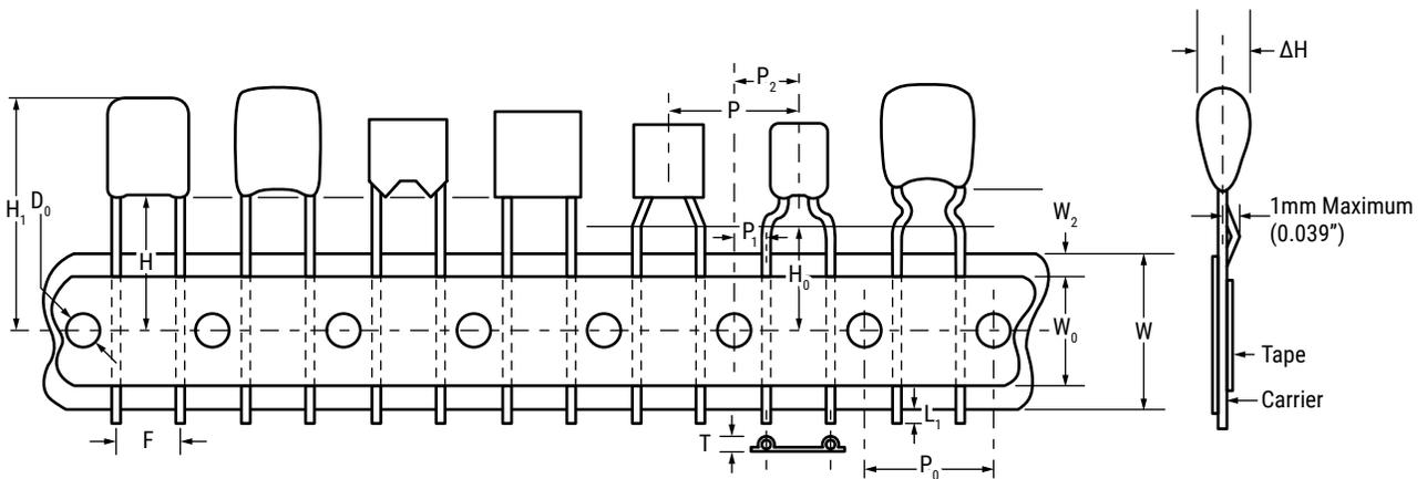
Figure 2: Lead Tape Configuration (See Table Below)
