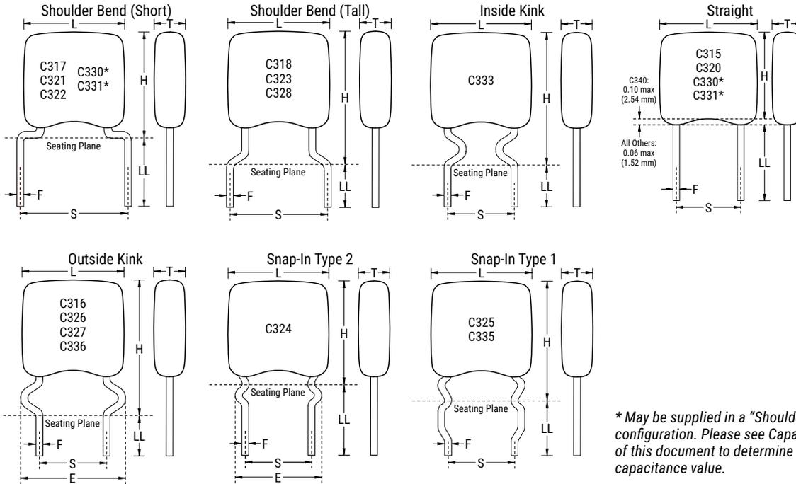
\* May be supplied in a "Shoulder Bend" or "Straight" Lead configuration. Please see Capacitance Range Waterfall section of this document to determine lead configuration availability by capacitance value.
