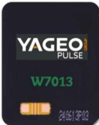
The W7013 is a flexible Near Field Communication (NFC) antenna ideal for tight-space embedded products such as tablets, laptops, printers and other unique system using NFC technology. It is intended for pairing and sharing modes typically found in non-payment NFC applications.
