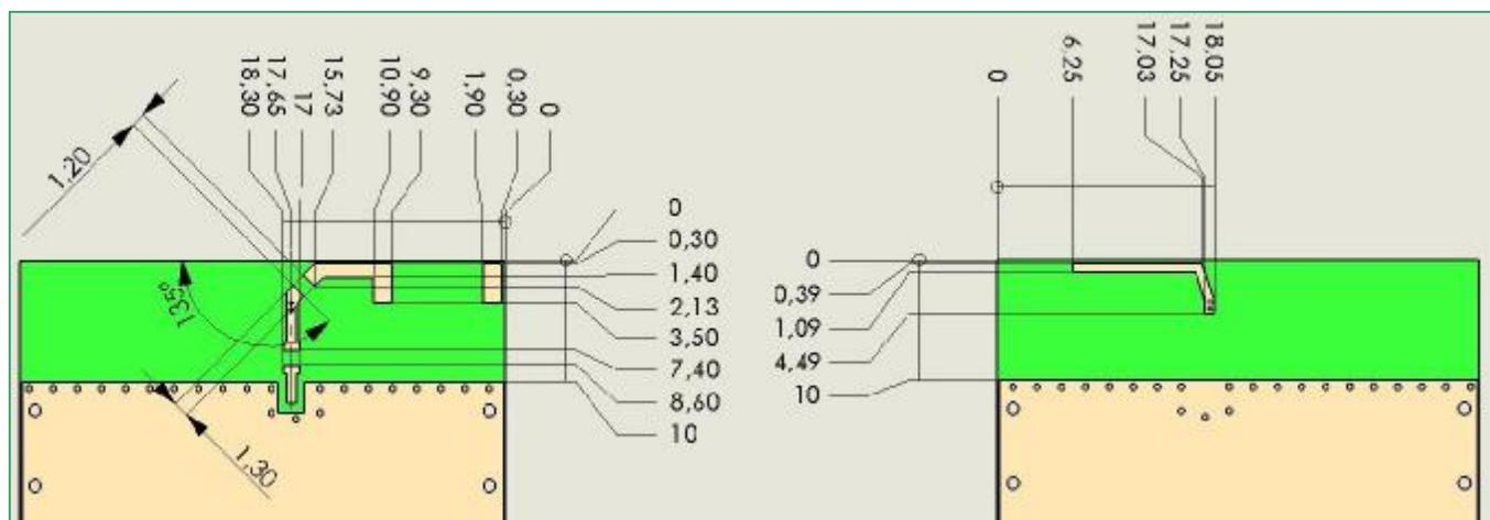
*Recommended test board- layout for electrical characteristic measurement. Test board outline size 95 x 40mm.*
