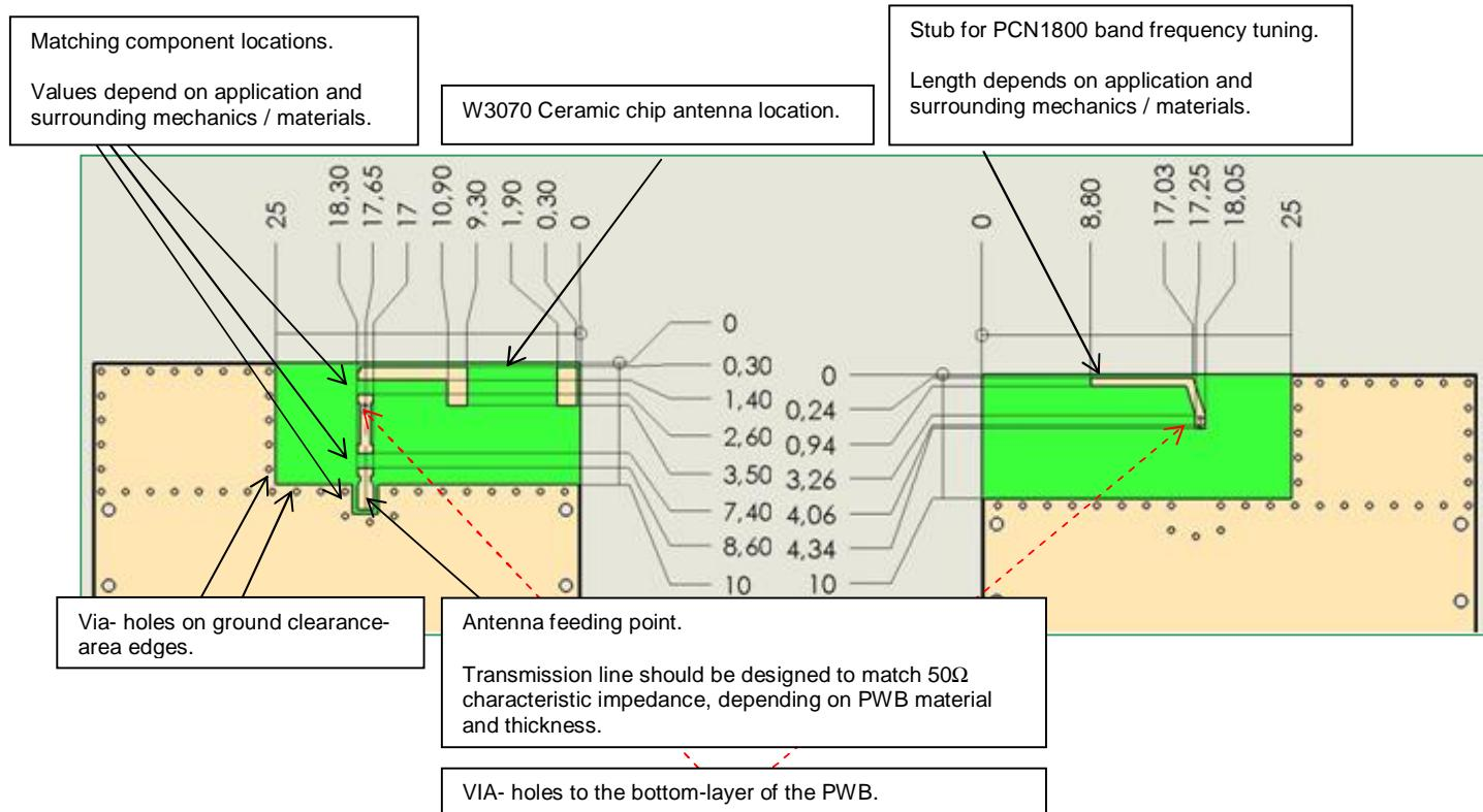
Ground cleared under antenna, clearance area **40 mm x 10 mm**
