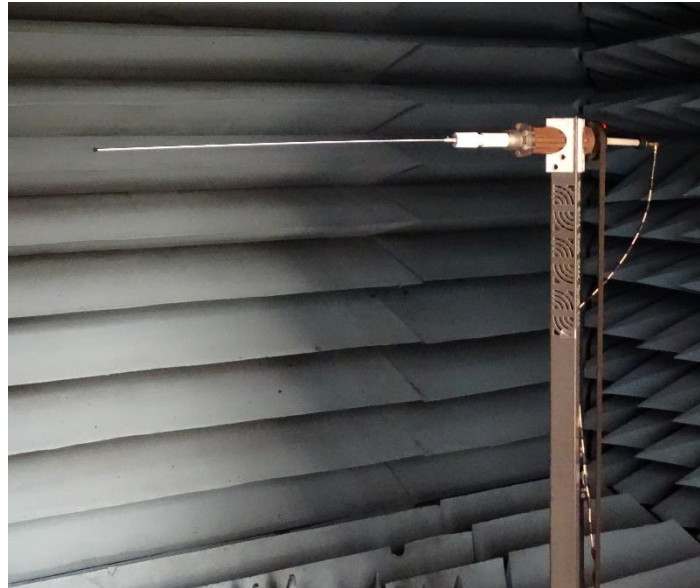
DM220C antenna sample measured in free space
