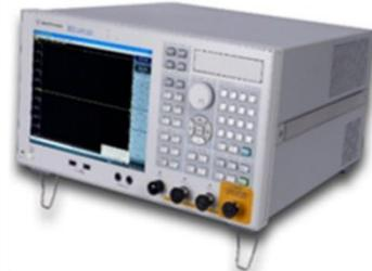
S11 measurements were taken with Agilent E5071C ENA, 9kHz- 8.5GHz
