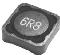
**1 Scope:** This specification applies to the Pb Free high current type SMD inductors
